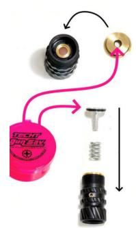
Grease the seals on the brass disk. Place the disk on top of black part with the external seal facing down.
