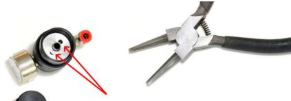
Use a pliers with rounded tips to unscrew (CCW) the steel regulation knob. There are a special holes at the bottom.
